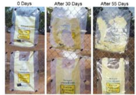
Illustration of photo and thermal degradation of a shopping bag incorporating EPI's TDPA® Additive (top row) vs. a bag without EPI's TDPA™ Additive (bottom row). Test procedures follow ASTM D5272 "Outdoor Exposure Testing of Photo Degradable Plastics" Guidelines.
